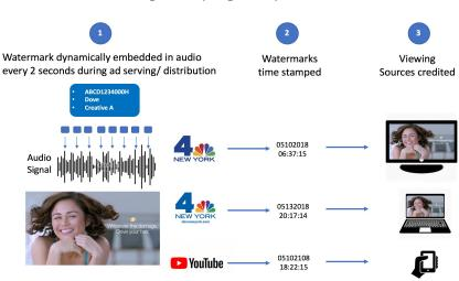
serving firms. The distribution ID is repeatedly inserted into the broadcast or digital stream every 28 seconds. Both TAXI IDs can be detected in hardware such as set-top boxes, Smart TVs, or meters attached to the TV. Detection can also occur acoustically via apps on portable devices, such as smartphones or tablets.
